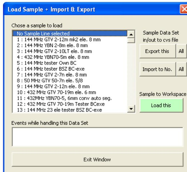
Scroll the data base, identify the design to be loaded into the workspace area and mark it. Upon clicking the 'Load this' button you will be asked whether to really load this sample or exit when the workspace is not empty.
