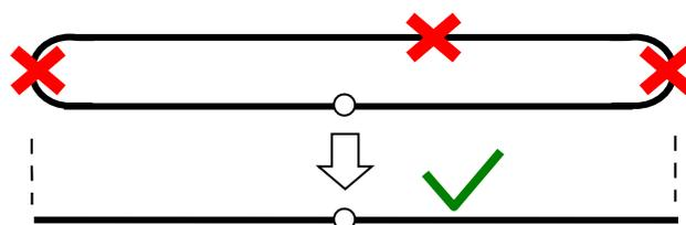
Remove all rows holding GW Cards that form the arced ends and upper arm of the folded dipole. Then prolong the fed wire to the original span width of the ex-Folded Dipole, measured on outer ends.
