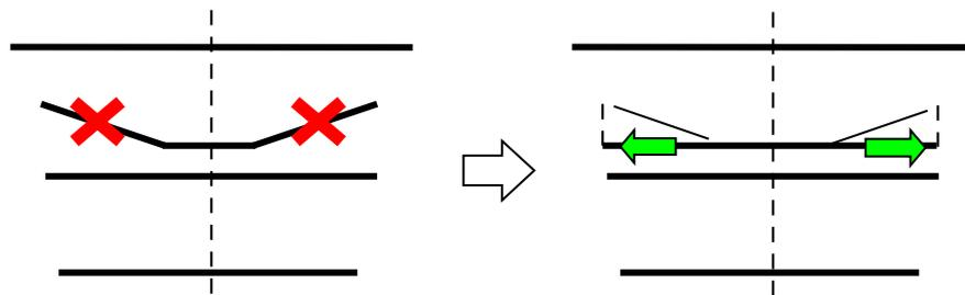
Example (2) LFA Loop : the “GW” lines holding the side arms and one of the parallel long wires must be deleted as entire rows on the MS Excel sheet. With just one wire or “GW” card line left the BC to be applied to the LFA Loop can be produced as if it still would be present in its complex structure.
