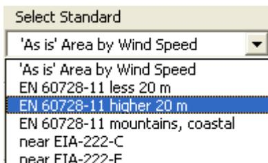
For “**EN 60728-11 higher 20 m**” a fixed Dynamic Pressure of 1,100 N/m<sup>2</sup> is used. So wind speed edit is frozen for this option
