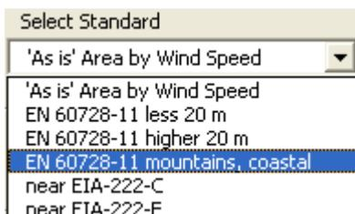
For “**EN 60728-11 mountains, coastal**” a fixed Dynamic Pressure of 1,250 N/m<sup>2</sup> is used. So wind speed edit is frozen for this option
