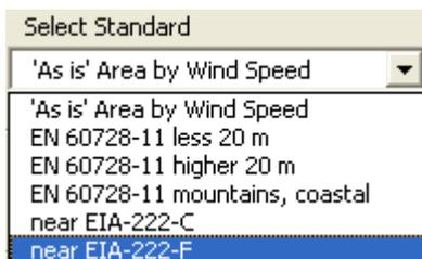
For “**near EIA-222-F**” a wind speed according landscape wind speed zone maps shall be selected. This standard uses a “**3 sec gust**” instead of fastest mile throughout. So any entered fastest mile wind speed is computed in to a referring gust speed. See next page for details.
