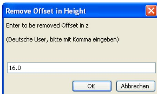
Clicking the button 'Remove Offset in z' brings up this little popup form here. Please enter the Offset that shall be removed. Attention, in here the decimal separator is sensitive.
