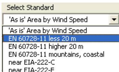
For “**EN 60728-11 less 20 m**” meaning antenna height below 20 m a fixed Dynamic Pressure of 800 N/m<sup>2</sup> is used. So wind speed edit is frozen for this option
